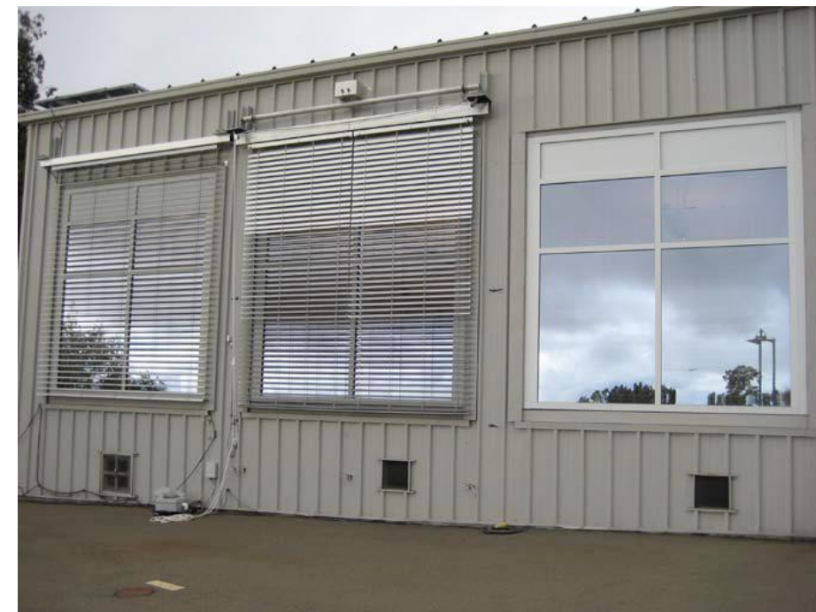
Exterior view of the LBNL Windows Testbed Facility with the VB-E1n and VB-E3opt systems installed on the left and middle test chamber windows, respectively. The reference case with an interior Venetian blind (reference-VB) is on the right-most chamber window.
